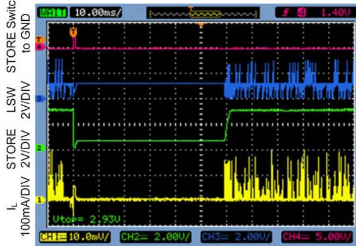
Short STORE to GND for 1msec Recovery : Circuit A V IN =1.2V, STORE=3V, I STORE =2mA
